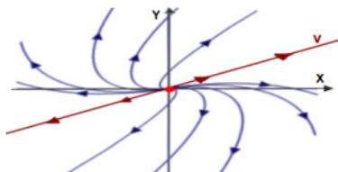
Figura 7.9: Nodo impropio inestable
